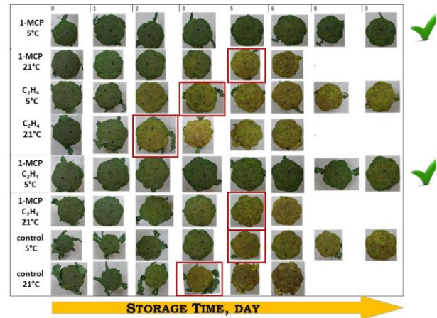
Fig. 2. Overall broccoli quality changes represented by the digital pictures taken during storage
