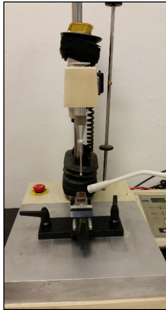
Figure 1. Set up of the acoustic measurements using SMS XT-2A
