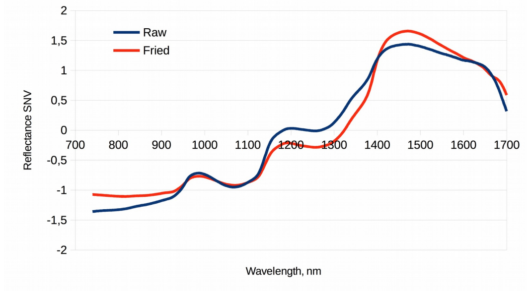
Figure 2: Standard normal variate of NIR spectra for raw (blue) and fried (red) samples
